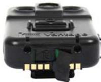
2. Insert and dock the Vantage unit into the Base Station in order to sync them together and to charge the BWC battery.
