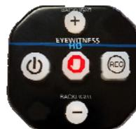
Your system has been configured to power on and off automatically with the vehicle's ignition, or you will control power with the small controller module pictured here. You will also need to open the EyeHD program on your laptop (usually an icon for the program is added to the desktop to make this easier). Bootup should take a couple minutes. Once live video is shown on the MDC display, the system is ready to operate.
