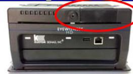
Before turning on the system, confirm that a media drive is loaded in the DVR. If not, insert the drive and lock it in place. If you remove the drive at the end of the shift (as opposed to using wireless file transfer), use the key to unlock the cartridge, then pull it out of the DVR and turn it in for ingestion into the database.
