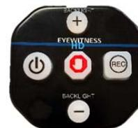
Your system has been configured to power on and off automatically with the vehicle's ignition, or you will control power with the small controller module pictured here. You will also need to open the EyeHD program on your laptop (usually an icon for the program is added to the desktop to make this easier). Bootup should take a couple minutes. Once live video is shown on the MDC display, the system is ready to operate.
