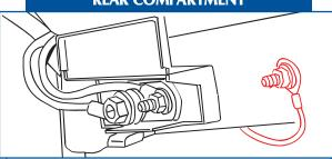
This feature provides a 10mm ground stud located in the trunk on the right side just above the red Trunk Auxiliary Battery Power Junction Block. A 10mm flanged hex nut grounds the 10mm stud bolt to the vehicle and is torqued to 26 lb-ft (35N-M). A plain 10 mm hex nut is provided for customer ground termination. Recommended torque for this second nut is 7 lb-ft (10N-M) plus or minus 1 lb-ft (2N-M).
