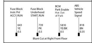
Bunt cut ignition controlled power and signal circuits are also included in the following 5-foot (1.5 m) right foot loop. The spotlamp fuses are located in the passenger's side underhood fuse block. See "Fuses and Circuit Breakers" in your owner's manual index for more information.
