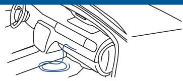
The vehicle is equipped with wiring provisions for connecting 12-volt battery power to customer installed equipment. Refer to the following information when adding electrical accessories that will use the 12-volt power supply circuits connected to the vehicle's electrical system. A wiring harness is located below the instrument panel (IP) near the center of the vehicle and another connection point is located in the left rear of the cargo area.
