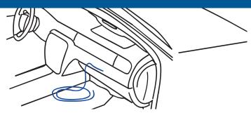
The vehicle is equipped with wiring provisions for connecting 12-volt battery power to customer installed equipment. Refer to the following information when adding electrical accessories that will use the 12-volt power supply circuits connected to the vehicle's electrical system. A wiring harness is located below the instrument panel (IP) near the center of the vehicle and another connection point is located in the left rear of
