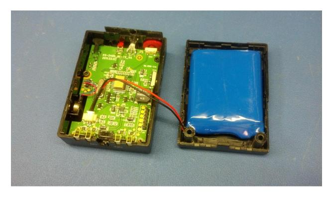
6) The new battery will have the same connector as the old battery so should connect to the PCB connector without issue. Please be careful not to pinch the wires when closing the case.
