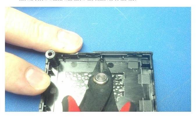
5) The new battery should then fit snugly in the new space after the 4 tabs are removed.
