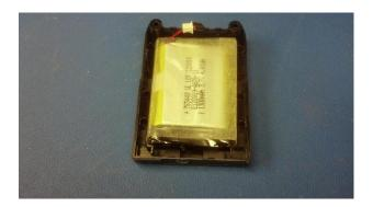
3) Take a pair of side cutters and remove the four side tabs that hold the battery in place as shown below. The new battery will not fit into this space unless these four tabs are removed.
